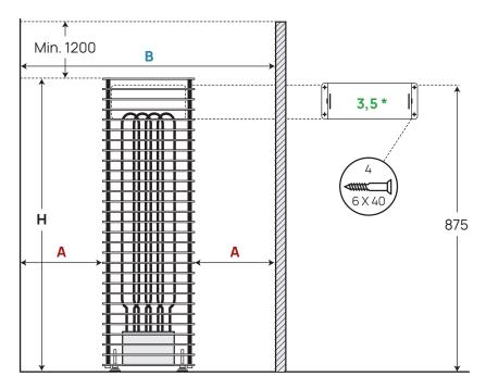
\* CLIFF Mini 3,5 is attached to the wall with a special bracket See CLIFF Mini 3,5 heater data in the table below.
