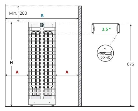
\* STEEL Mini 3,5 is attached to the wall with a special bracket See STEEL Mini 3,5 heater data in the table below.
