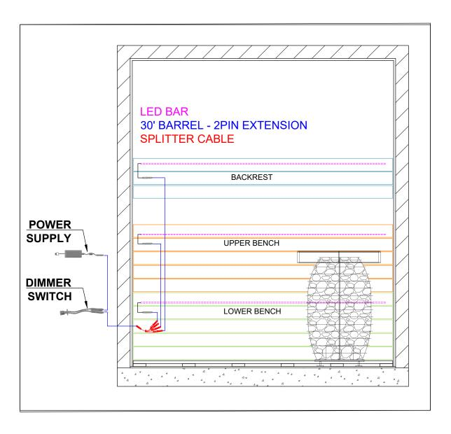
**Figure 5: Connections Diagram 2**
