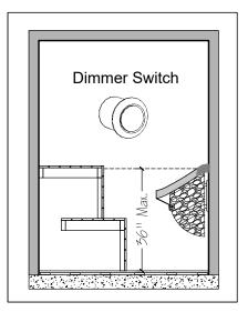
Figure 7: Dimmer Switch Location Elevation View
