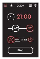
While the sauna is in heating mode, it is possible to change the "sauna ready" time and the temperature by tapping on the time and temperature controls and selecting the desired numbers.
