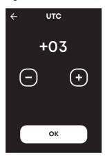
The local time zone (UTC) configuration is required if the sauna control panel has been previously connected to the Wi-Fi network.
